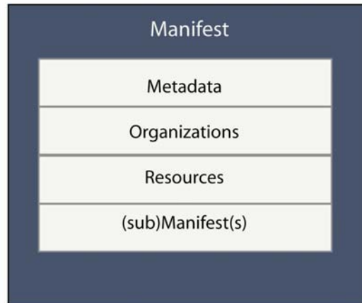
Figure 3.3a: Components of a Manifest
