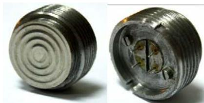
The photo on the left are thin-film sensor protected from exposure to environmental metal separation membrane made of stainless steel 316L. The pressure is transmitted through the organ silicon fluid that lies between the sensor and the membrane. This sensor can be installed in any building, or used independently. The sensor is resistant to gamma and neutron radiation.
