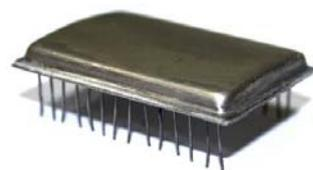
Multi-point measurement module combines, in this case, 12 silicon tensoconverters in a single package and allows you to carry out simultaneous measurements at 12 points.
