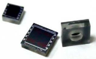
Sensors are equipped with modern silicon MEMS tensoresistive sensors that have a high overload capacity of 100 - 150 times exceeding the upper limit of measurement. The photo on the left are the Silicon tensoconverters of pressure, coupled with the glass marks "Pyrex" by electrostatic welding.
